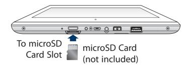
Insert the microSD card into the tablet's microSD slot until it clicks.
